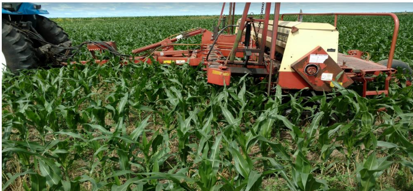
Interseeding cover crop into corn using a modified no-till drill planting cover crops between 30" corn rows. (Photo credit: Grass Fed Insights)
